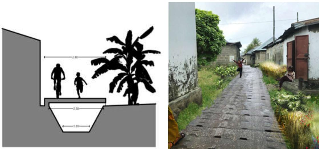
Figure 2. 7. Green Link cross section
