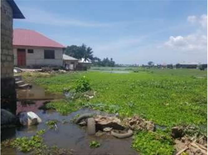
Spot located at Meya Magomeni, in which Storm water flows together with solid wastes leading to clogging of underground channel and leads to flooding.
